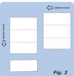
Figure 3 shows one of the most popular ways to get a big increase in folding machine yield. Here you run a letter-fold or 6-panel job 2-up. Apply 2 creases in the first section (no folding.) In the right angle section, fold 2 times, then take a trim out of the middle using a premium cutting tool such as Technifold's Multi Tool to yield 2 pieces. With the Multi Tool, you can even do this on cover stocks since you are getting guillotine quality cutting.
