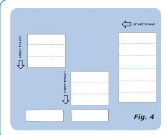
**Figure 4** illustrates a **technique for running a 2-up job**. Typically (but not always) this requires a split guide on the right angle section. If you do any long runs and a split guide attachment is available, it's well worth the investment since production increases can be huge.
