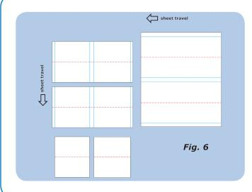
Figure 6 demonstrates another inventive use of multiple Technifold tools to get a huge increase in yield. Here a 4-up 11.5 x 15.5" sheet is taken directly from the press (no trimming,) creased, trimmed and delivered flat.
