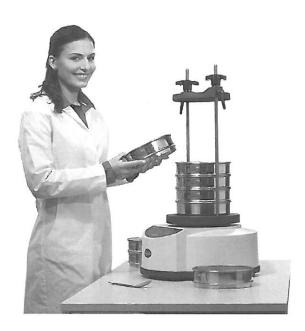
The sieve set is made up of the collecting bottom and the analytical sieves, which are arranged one on top of the other according to increasing mesh size and a the final lid.
