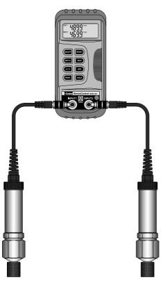
Calibrate the pressure sensors at the operating pressure of the machine.
