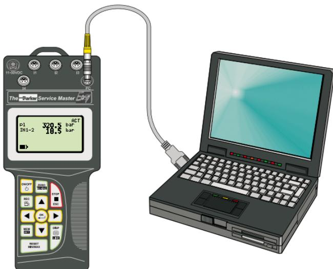
Measuring instrument, PC and USB cable
