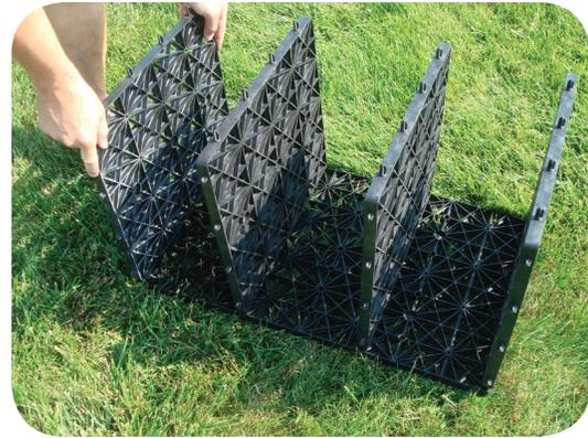
There are seven rows of holes for setting the support panels. Push the four end / center panels into place utilizing the two end positions and the two rows located on either side of the center position. Be sure you insert the long tabs at this stage leaving the short tabs facing to the sides.
