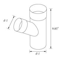
24 Guage Zinc Magnesium Steel and sprayed with a proprietary scratch and fade resistant paint.
