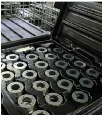
Reusable Static Intercept Trays enables the manufacturer to use their own standard size shipping crates. The inserts are designed to fit into the existing reusable packaging and allow for Corrosion and Static protection without the use of oils or volatile inhibitors.
