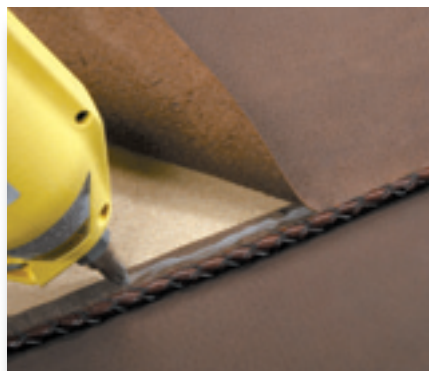
For furniture and upholstery, PUR 250 adhesive bonds leather or fabric gimping and seams.
