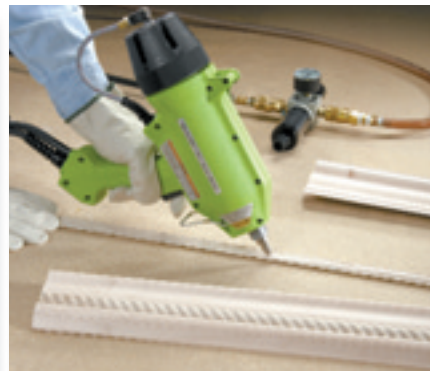
19 For both PUR Easy and PUR Easy 250, an optional filter/pressure regulator is available to remove particulate material and water.
