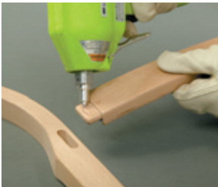
18 Adhesives are available for bonding a variety of wood sizes and configurations such as this mortise and tenon assembly.
