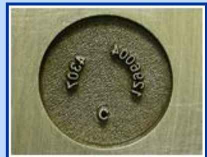
Laser Scribing on concave surface with vision system
