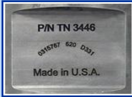
Z-axis with Auto-Focus for Laser Focal Length, 5x6 matrix, parts with multiple height
