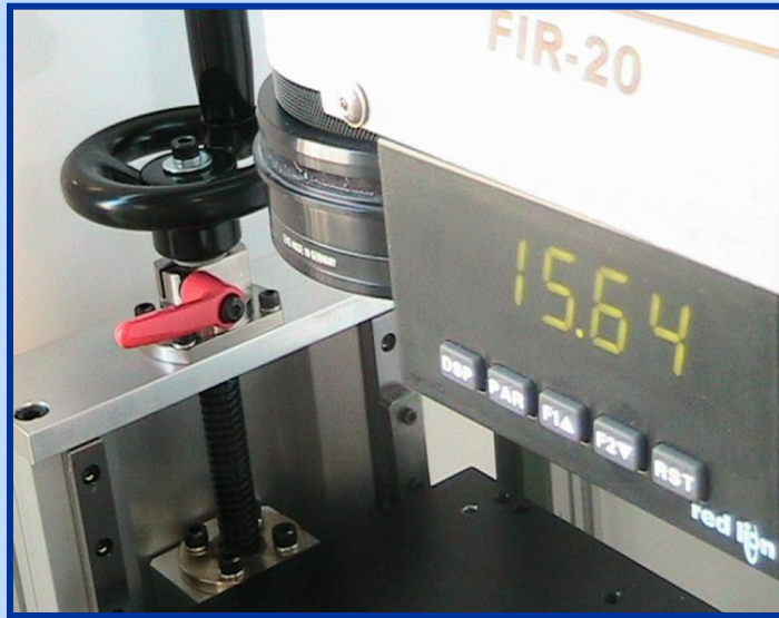
Laser Machine with manual Z-axis and digital display
