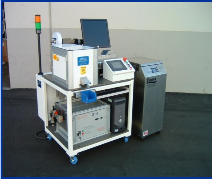
Label Marking w/Auto-feed, Programmable Cut-to-length unit and Fume Extractor.
