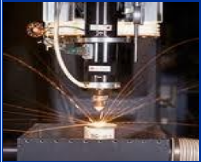
Laser cutting with Nitrogen assist for clean & deep cutting & Micro-machining
