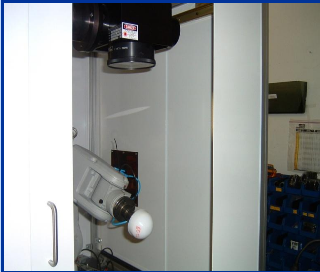
6-Axes Robot Handling Medical Implants for Contrast Laser Marking on UHMWPE
