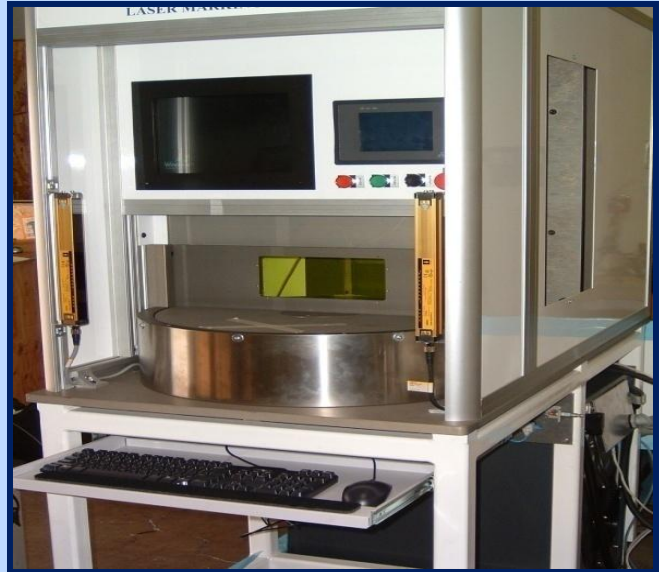
Laser Machine with Precision Index Table for higher thru-put
