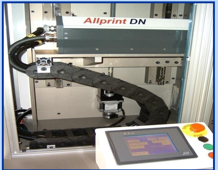
Laser Work Station with programmable Z-axis for focal length adjustment.
