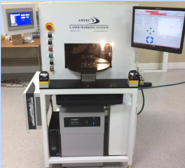
Laser Marking System w/Rotary Index table for higher production capacity.
