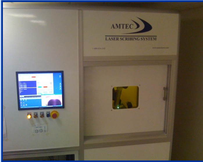
Laser Work Station with Fixed Beam Delivery and 5 axes Part Handling System
