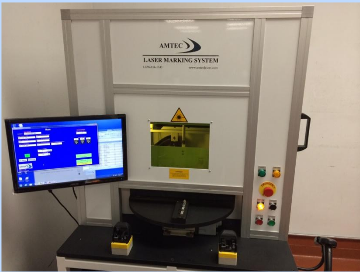
Laser Work Station: 3 Marking Heads integrated with 1 laser source
