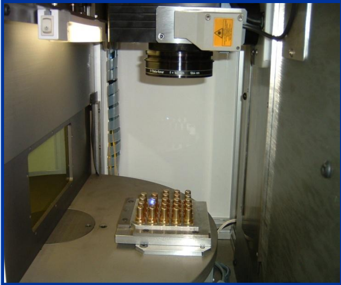
Z-axis with Auto-Focus for Laser Focal Length, 5x6 matrix, parts with multiple height
