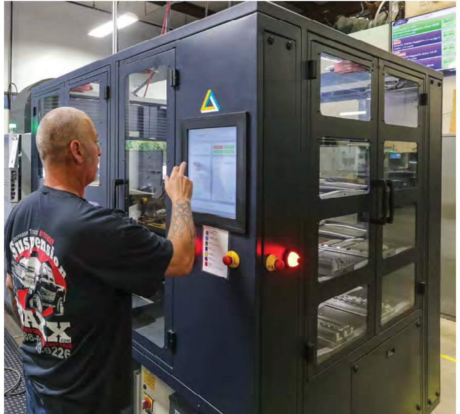
PNM just added a new Trinity robotic cell system attached to a Haas VF2ssYT with 42 tools. Mario estimates that with all 56 pallets populated that they will net 12-14 hours of run time with only three man hours of labor. PNM considers Mexico and China as their biggest competitors so any time they can see long production runs with low labor interaction they are very happy. Pallets, technology, robots, and automation keeps them competitive.
