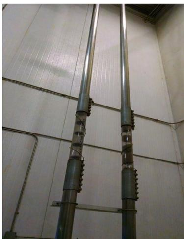
Apffels is the most state-of-the art automated coffee roasting facility in the world. From roasting, to blending, to packaging, the coffee is transported through air-tight conveyor tubes with no human hands ever touching the coffee! Also see the conveyor tubes in the photo on the right.
