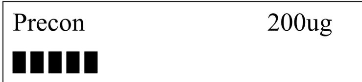
This screen indicates the instrument is preconditioning, (removing excess moisture from the cell). The Aquapal will go into preconditioning when power is applied with the cell switch on or when the cell switch is turned off then on.
