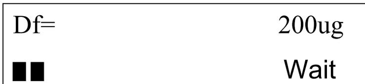
After preconditioning the Aquapal starts to calculate drift in ug per minute.
