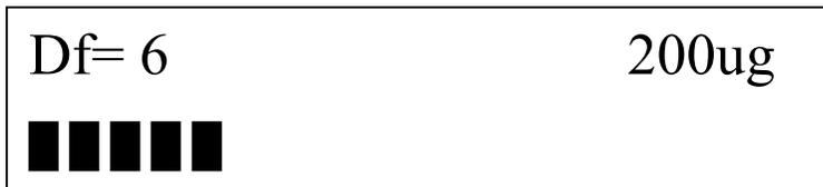
This display shows the Aquapal running a test the ug count will increment and the detector indicator bars will reduce as the test Progresses to the end point.
