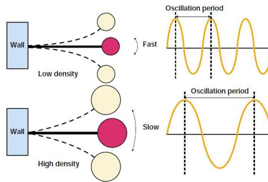
When the measuring is vibrated in a chamber filled with liquid or gas, its oscillation frequency differs from density of sample.
