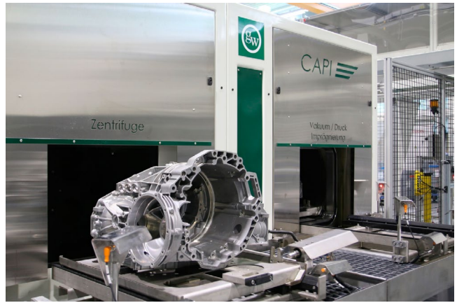
Figure 3 - The CAPI's single piece flow ensures all 1,500 machined features are free of contamination.
