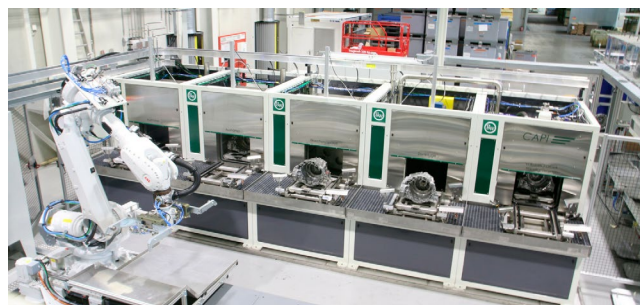
Figure 1 - The CAPI is a fully automatic impregnation system that enables manufacturers to bring vacuum impregnation in-house.
