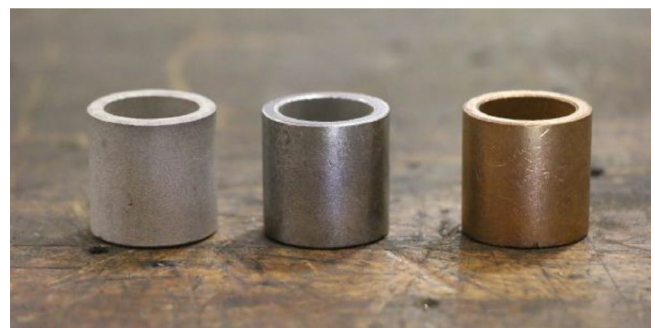
Figure 1 - The test ring shall be 1 inch (25.4mm) long with a nominal ¾ inch (19.0mm) inside diameter and 1 inch (25.4mm) outside diameter.
