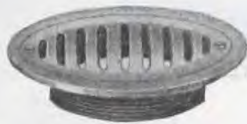
No. 94 Brass N. P. or polished Benedict nickel. This strainer is made in two lengths, 2 and 4 inches, and with either a flat or beehive strainer. Diameter of top 5½ inches. Made with 3-inch standard iron pipe thread.
