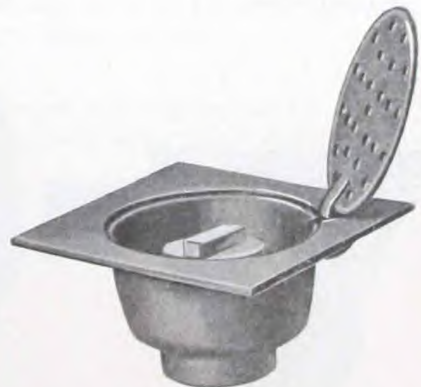
No. 863-B Plenum Chamber Drain Iron body, depth 4½ inches. Diameter 9 inches, with iron strainer or all-brass top with hinged strainer. Outlet fitted inside with 3-inch brass plug with oblong raised head.
