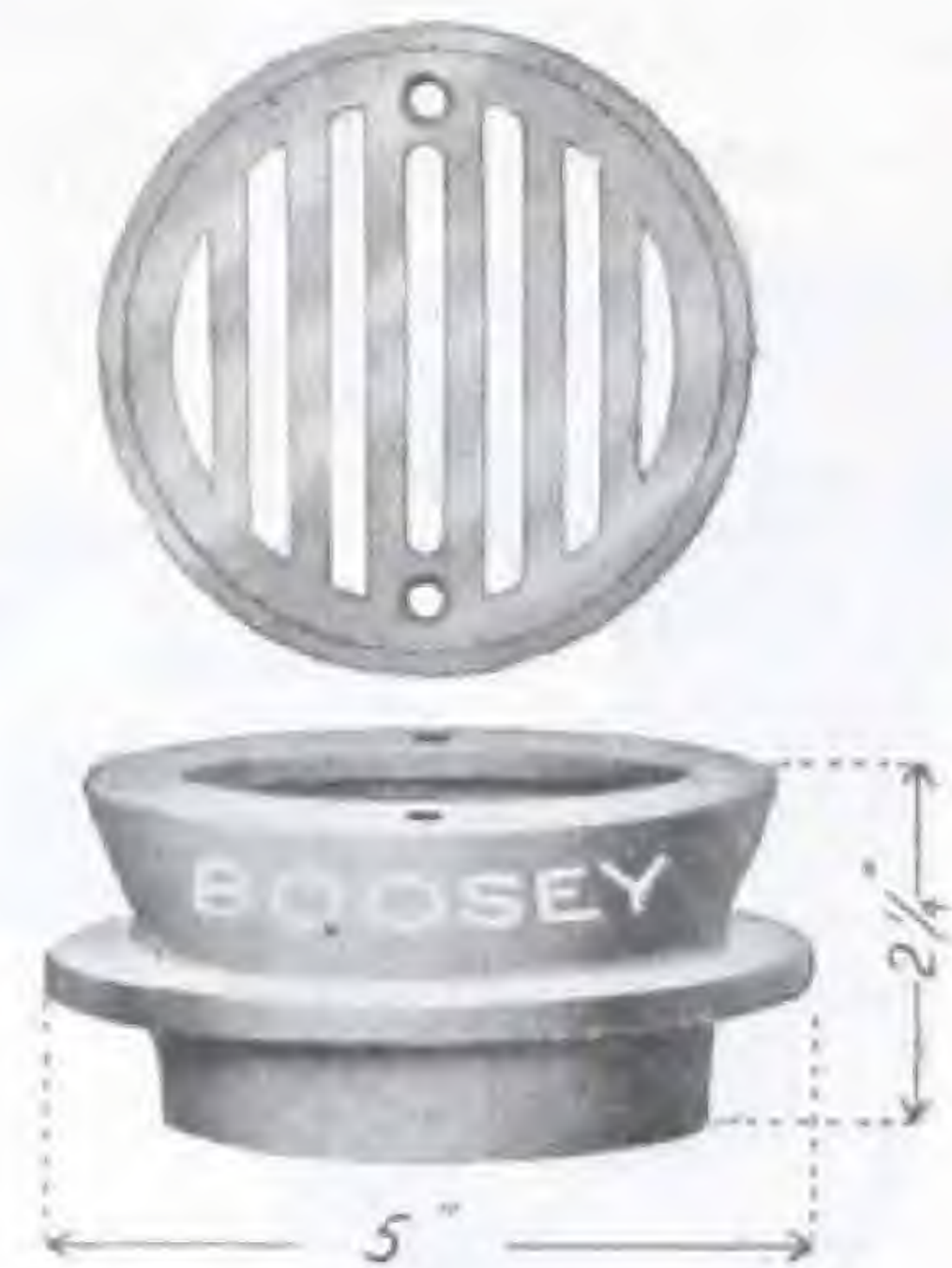
No. 91 Brass N. P. strainer and ring. Body cast iron. Tapped 2-inch standard iron pipe, female.
