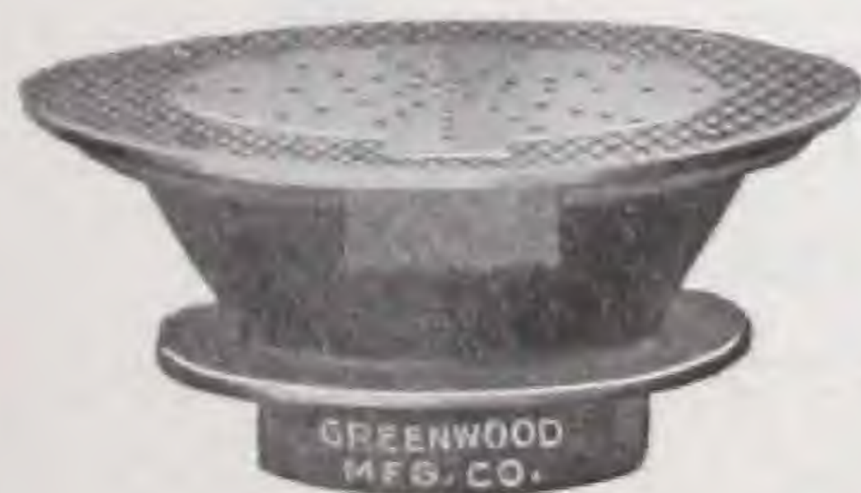
No. 92 Floor Drain Iron body tapped 3 inch, female. Depth 4 inches. Fitted with 9-inch finished brass top, with hinged strainer secured to iron body with brass screws. Also furnished in polished Benedict nickel.
