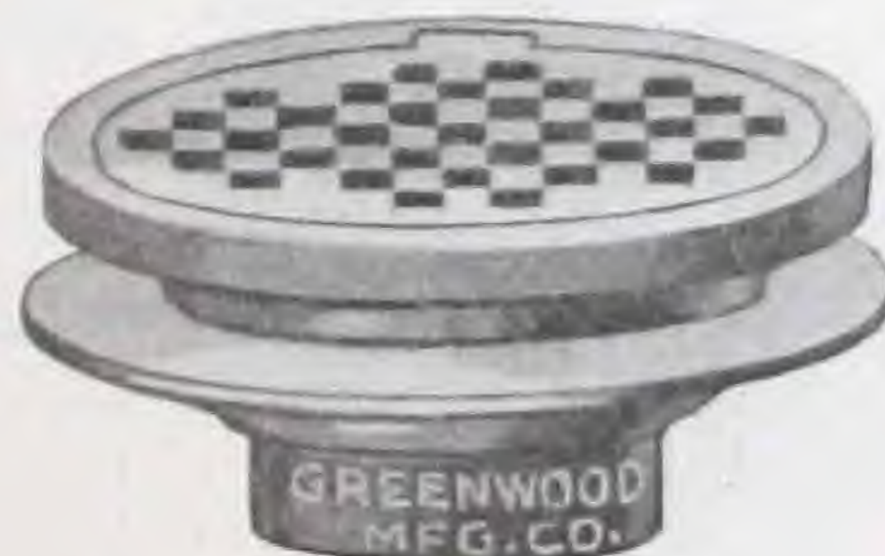
No. 96 Factory Floor Drain Iron body tapped 3 inch, female. Diameter 8 inches, depth 4 inches. Fitted with iron or brass strainer ½-inch thick, hinged to body with brass bolt.
