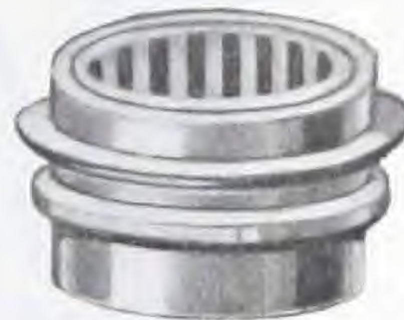
No. 124 Brass N. P. strainer and ring. Body cast iron. Tapped 3-inch standard iron pipe, female.
