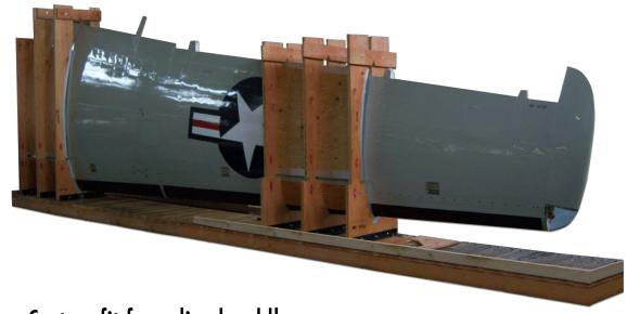
Custom fit foam-lined saddles connect directly to the containers base, protecting against vibration & abrasion during transit.
