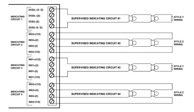
NOTES: ALL CIRCUITS ARE POWER LIMITED, AND MUST USE TYPE FPL, FPLR, OR FPLP POWER LIMITED CABLE. INDICATING CIRCUITS ARE FULLY SUPERVISED AND RATED FOR 24 VDC UNFILTERED 1.7 AMP MAX. THEY MUST BE WIRED AS SHOWN IN THE WIRING TABLES.
