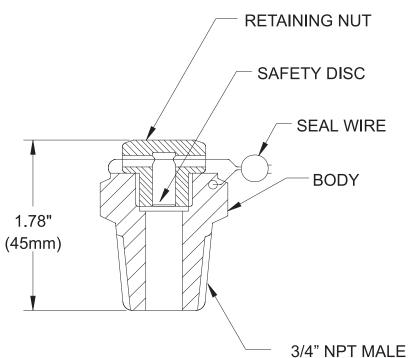
MATERIALS BODY AND RETAINING NUT: BRASS SEAL WIRE: COPPER AND LEAD
