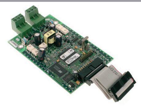
The VESDAnet™ Interface Card (VN Card) is a simple interface card for the range of Xtralis VESDA VLF smoke detectors. The VN Card provides seamless VESDAnet communication from the detector to other VESDAnet devices, including configuration and monitoring tools.
