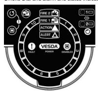
When the field service access door is open, the user has access to the RESET C DISABLE , Fire Test , AutoLearn and Instant Fault Finder functions. When the Instant Fault Finder function is activated, the Smoke Dial converts to a fault indicator, with the dial segment numbers corresponding to the faults listed below.
