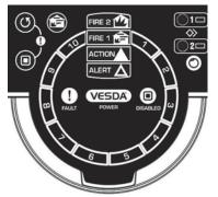
When the field service access door is open, the user has access to the RESET (J DISABLE , Fire Test 1 , AutoLearn and Instant Fault Finder functions. When the Instant Fault Finder function is activated, the Smoke Dial converts to a fault indicator, with the dial segment numbers corresponding to the faults listed below.
