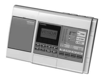
The Xtralis VESDA VLP detector is the central element of the Xtralis VESDA ASD product range. Using unique detection principles, the VLP has an alarm sensitivity range of 0.005%–20% obscuration/m (0.0015%–6.25% obscuration/ft). The VLP is classed as a "Very Early Warning Smoke Detector", which means that it detects fire at the earliest possible stage and reliably measures very low to extremely high concentrations of smoke.
