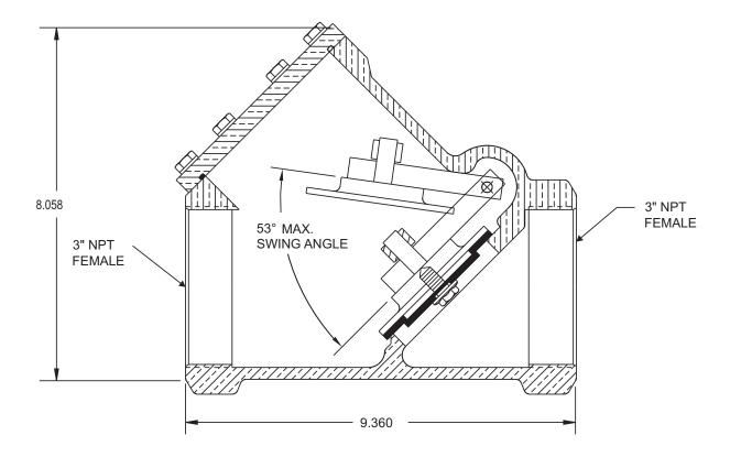
**Note:** The valve must be installed with the arrow pointing in the direction of flow.
