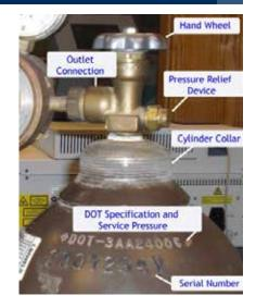
The common denominator, however, is that the gas contents are under pressures up to 2,500psi. This presents an inherent hazard
