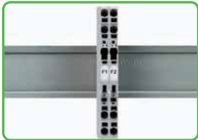
Fuse terminal blocks with a width of 6.2 mm/0.244 in can be assembled adjacently. If there is no adjacent fuse terminal block at the end of the assembly, an end plate must be used.
