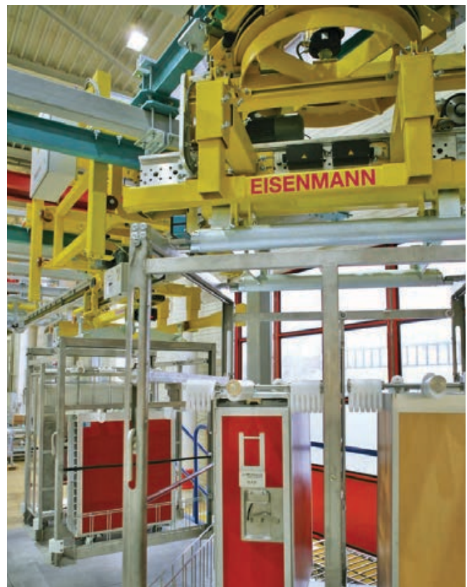
Turning stations at workstations enable direct access on both sides of the hanger.
