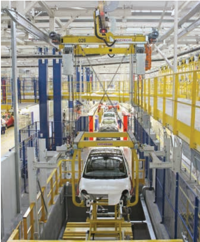
The chain lift provides flexibility in lifting and lowering of car bodies at workstations.
