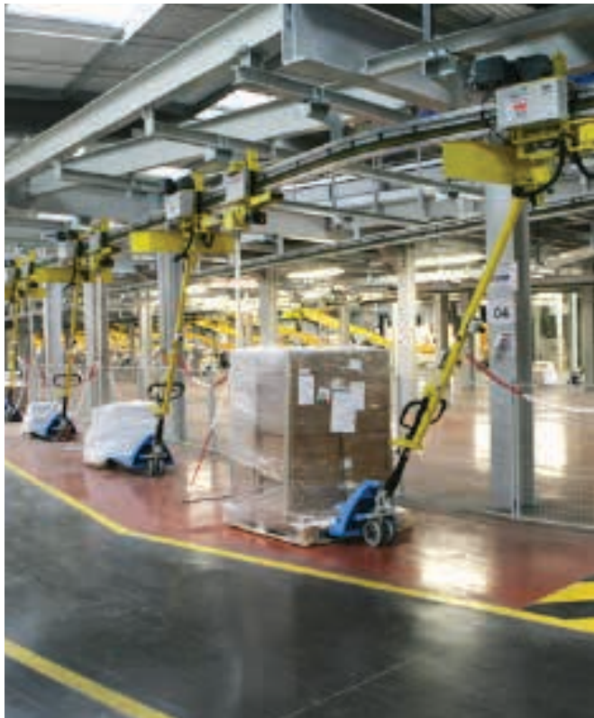
The VarioTow EMS combines the high performance EMS system with conventional pallet trucks.
