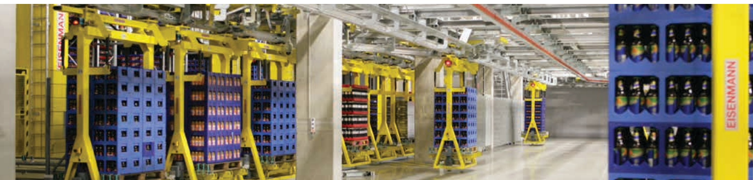
The EMS is a fast, intelligent conveyor that enables high throughput – making it popular with beverage manufacturers.
