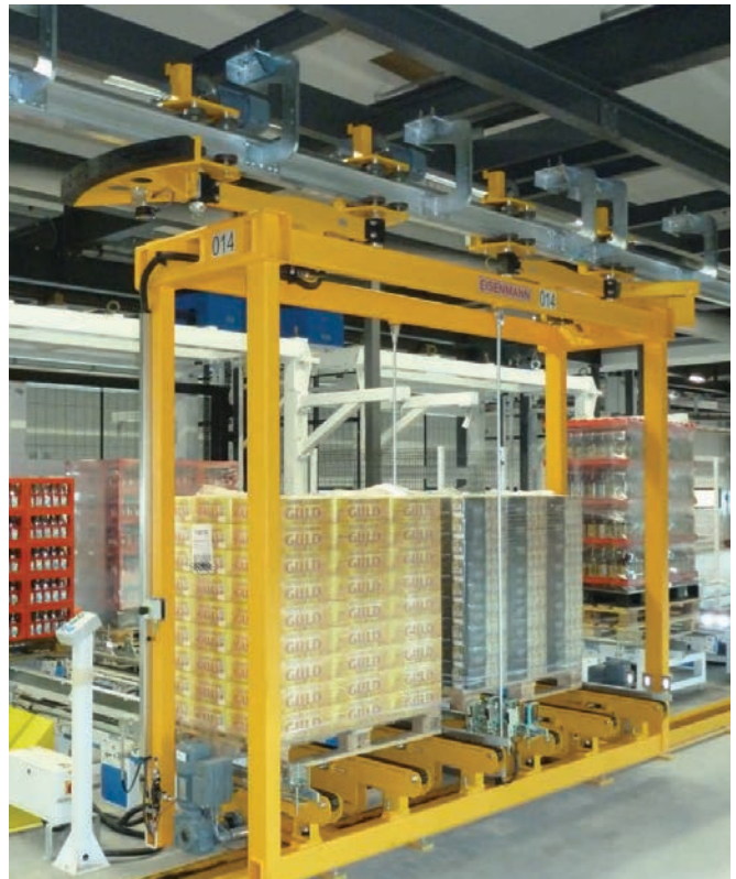
High throughput thanks to parallel pallet transfer.
