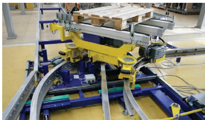
Sophisticated switching technology allows trolleys to be directed to branches without braking or stopping.
