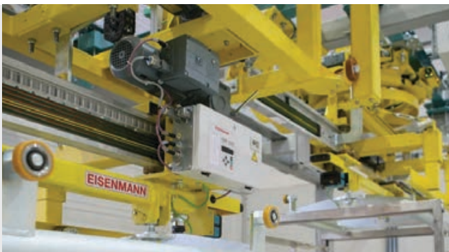
Plug-in trolley components are easy to replace.
