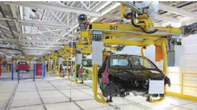
Thanks to its compact design, the chain lift is the ideal choice where ceilings are low.
