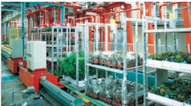
Automated handling of roller containers with our floor-based conveyor system.
