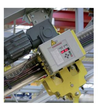
Mono-trolleys are perfectly capable of automatically mastering gradients when carrying payloads of less than 100 kg.
