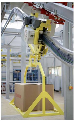
On duplex trolleys with front and rear trolley, the pressure unit is mounted on the front trolley.
