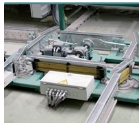
Quadro switch point with the advantage of space-saving design
