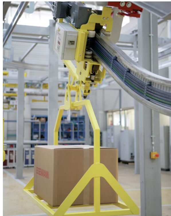
Electric monorail test course for practical trials and commissioning
