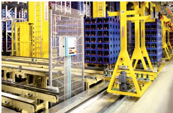
Floor guidance at transfer points ensures stability when loading
