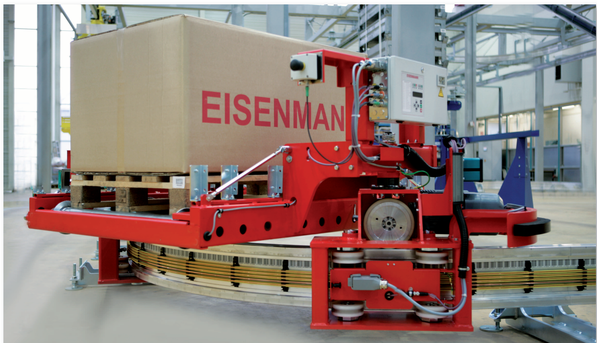
The new inverted electrified monorail system at the EISENMANN Conveyor Systems Test Center
