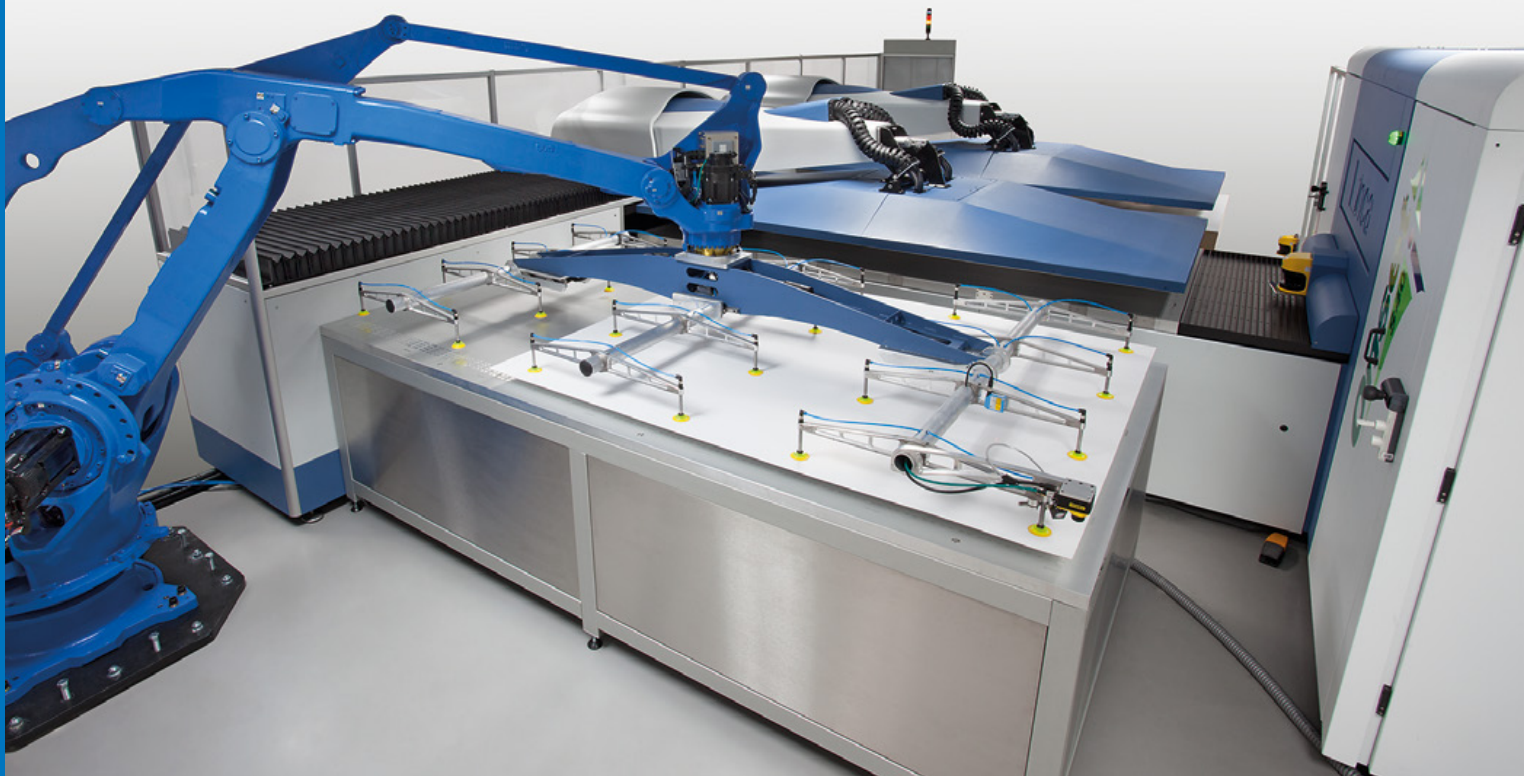
Fully automatic handling for unconditioned corrugated board
