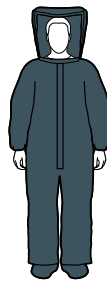
C3T450, Level B Encapsulated suit, rear entry, expanded back, 48" zipper, storm flap, 20 mil PVC face shield, elastic wrists, 2 exhaust ports with shroud, attached sock boots with boot flap. Suit is not gas/vapor tight. Sizes: S – 5XL Case Pack: 1
