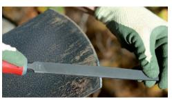
General purpose files for shaping steel or restoring sharp edges and where a smooth finish is important. Ideal for sharpening tools such as loppers, hedge shears, pruners, knives, spades, shovels, hoes, scrapers, etc. Good for polishing and deburring work on lathes.
