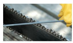
For sharpening cutters of saw chain.
