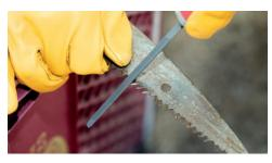
For sharpening conventional saws blades with fine universal toothing. Ideal for sharpening saws with 60° angle saw teeth. Tapered point to file tight angles.
