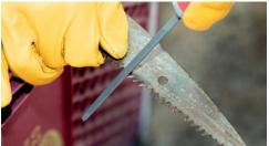
For sharpening crosscut saws, circular saws and saw teeth with less than 60° angle.
