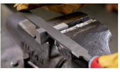
General purpose files for rapid removal or shaping of steel. High removal rate file for filing flat surfaces, sharp corners and shoulders as well as for deburring.
