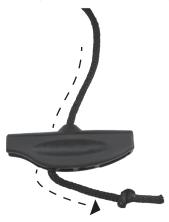
Pull rope against handle until rope can go inside of handle as shown on this picture:
