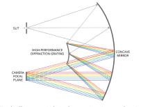
Headwall's concentric design layout using mirrors and gratings provides aberration-free imaging and a wide field-of-view.
