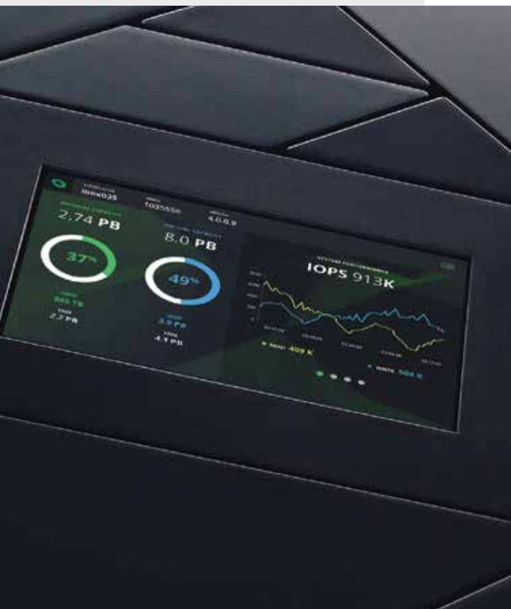
CONTROL PANEL OF AN INFINIBOX F6280 SYSTEM, CONFIGURED WITH 8 PETABYTES OF CAPACITY AND SERVING 913,000 IOPS PER SECOND.
