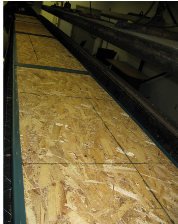
+ At right: Wall pads are placed horizontally and aligned end-to-end for an ASTM E84 tunnel test.
