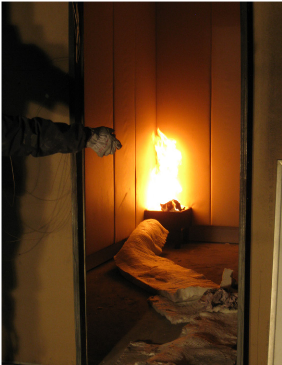
+ At left: An NFPA 286 large-scale room test is performed on a wall pad assembly, configured to match end-use conditions.
