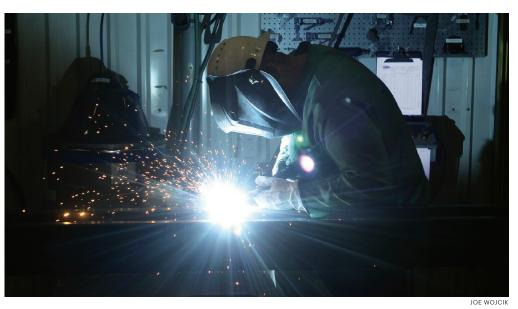
Mike Taylor welds a scissor arm using a process that utilizes metal inert gas and an electricity arc at Miller Welding & Machine Co. in Brookville.
