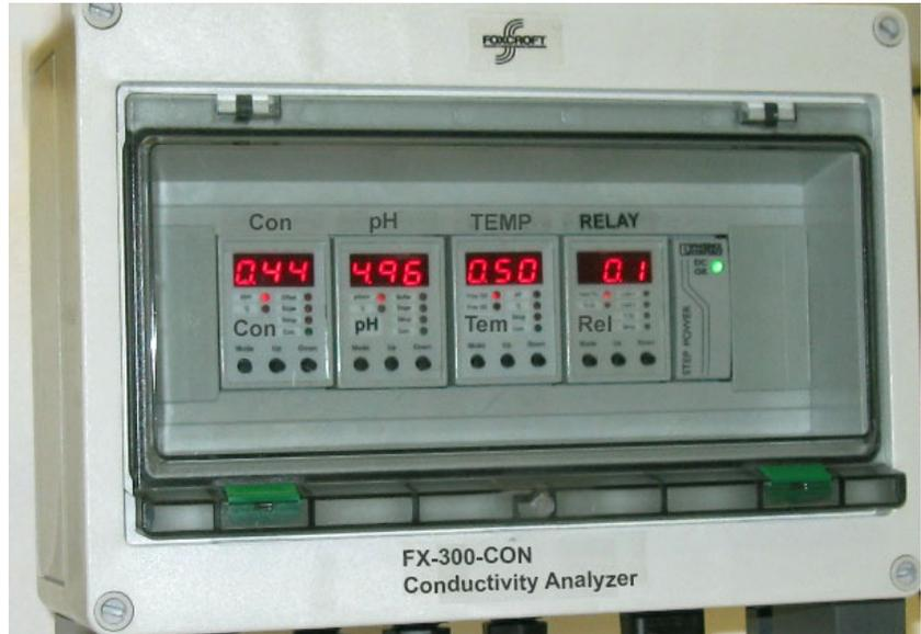
Shown: Conductivity, pH, temperature output with relay control of temperature
