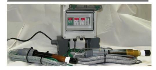
The heart of any fluoride removal or etching control system is the fluoride and pH sensors used to monitor the process.
