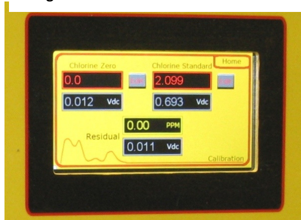
View Last Calibration Values & Live Readings During Calibration
