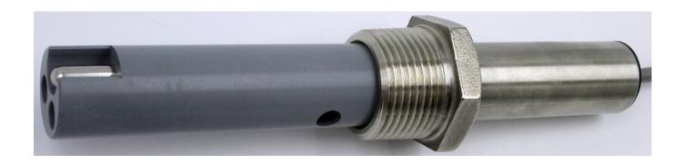
The sensor shown above has 316SS electrodes and sensor body with CPVC insulator. The 316SS electrodes are not visible as they are located inside of the two bored holes that go along the length of the insulator and are purged by the two corresponding vent holes on each side. The exposed 316SS thermowell is, however, visible which provide for fast temperature measurement to ensure accuracy conductivity values at any process condition.
