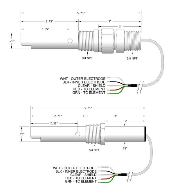
Drawings show configurations without the waterproofing option. Please inquire to factory for overall sensor length and dimensional details if the waterproofing option is needed.
