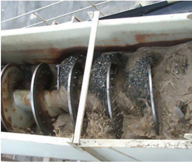
Figure 2) Top View - Coarse Material Screw Washer paddles in the feed area wash gravel contaminated with mud.
