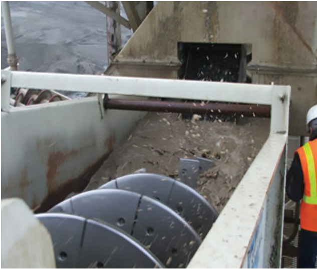
Figure 1) Rear View - Coarse Material Screw Washer paddles in the feed area wash gravel contaminated with mud.
