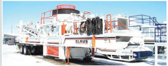
Chassis's for Most Cone & Impactor Crushers 1560 Omnicone® on 16 Wheel Suspension (Above)
