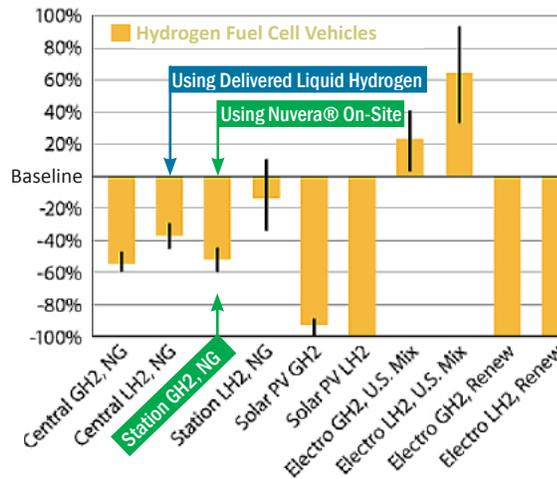
Generation of hydrogen on-site from natural gas and used in a fuel cell vehicle results in 45-60% fewer greenhouse gas emissions than a gasoline car.
