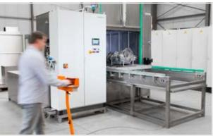
If your product range is very varied or changes, your cleaning processes need to be flexible too. Cleaning requirements can change from tool to tool or depending on customer contract. For this reason, we provide modular equipment to cover a broad range of tasks. Various types of ultrasonic, spray cleaning or drying baths can be linked together to form a modular cleaning unit. This is how we create custom cleaning solu-tions for our clients.
