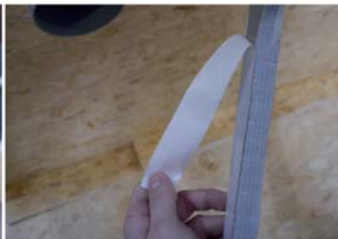
Remove the first sheet of silicone paper
