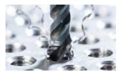
For this reason, primarily HSSE and HSSE-PM cutting materials are used for screw taps. These cutting materials can work with all material groups except hardened materials. Solid carbide is only used as a cutting material in a few tapping applications.
