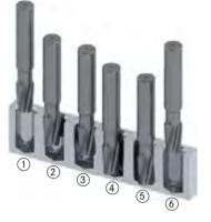
The multi-range thread milling cutter with collar recess is suitable for universal application. The collar recess enables very deep threads to be milled. With this type of cutter, all thread sizes can be produced at the same pitch above a nominal dimension.
