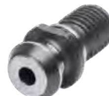
For Mazak4001 CAT metric SK40 with recess Ø6mm hole for internal cooling, with O-ring
