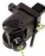
Drilling and milling head adjustable through 0°-90°
