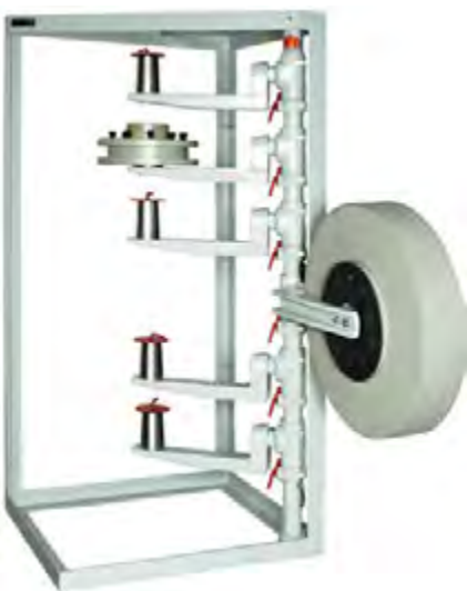
Sanding discs are tipped down and back with little effort as the discs are mounted exactly on their centres of gravity.
