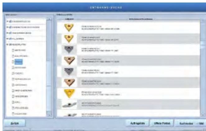
find the desired tool quickly using a simple search function. the software provides an overview of the tool stock and automatically triggers orders.
